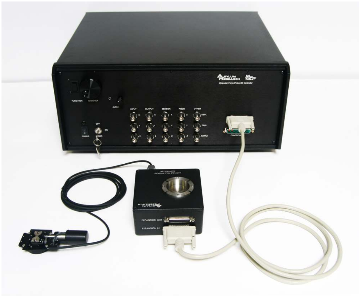
Figure 10.2.: The VFM sample stage plugs into the 9-pin connector on the VFM controller box. This in turn plugs into the 25-pin expansion connector on the front of the MFP-3D controller. This photo shows the older MFP-3D controller. The newer ARC2 controller can be used as well.
