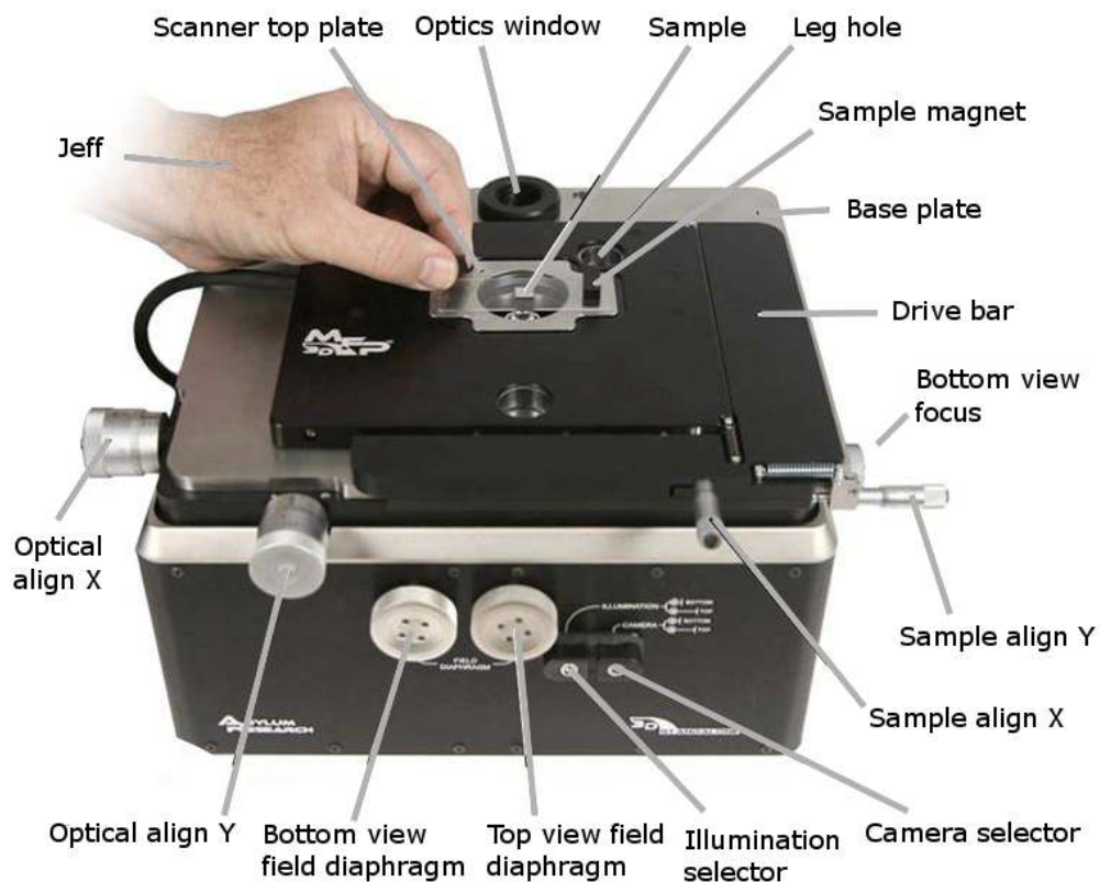
Figure 2.4.: Controls on the SA Base. Missing from view are (on the left) the aperture diaphragm which is a knurled ring around the entry point of the fiber optic illumination and (on the right) a large knob for focusing the bottom view objective.
