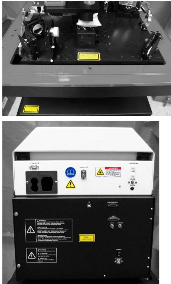
Figure 7-1 Locations of Laser Safety Labels
