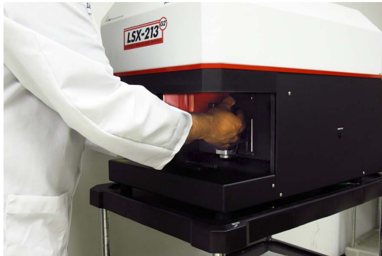
Figure 2-11 Lowering the Shield
